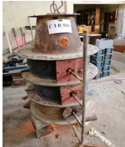
Fig.5. Columns subjected to fire
